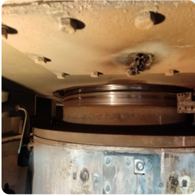
Undercut and uniform the Upper and lower portion of Bowl hub sealing portion Using spm mechanism.
