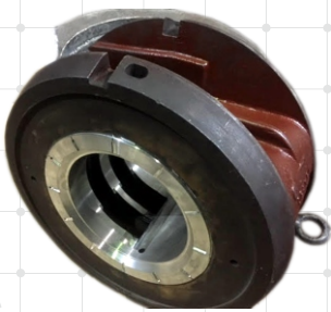
Rebabbiting of White Metal Bearing
